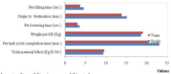
Figure 4: Impacts of team lifting in concrete lifting tasks
